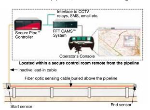
then digitally processed to identify and eliminate environmental nuisance alarms. Only real intrusion events are identified and security staff alerted.
