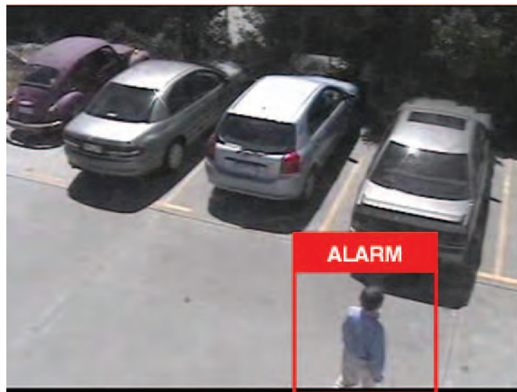
Intruder appears and is recognized by the change in the image and the behavior of this change, an alarm is set, intruder tracking and recording begins
