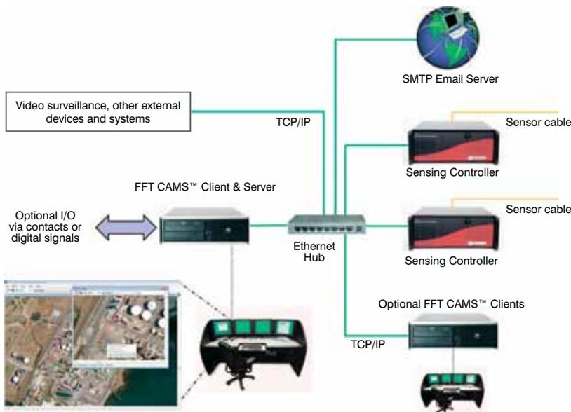
FFT CAMS™ seamlessly integrates intrusion detection systems with video surveillance, third party devices, as well as high level security management and access control systems.
